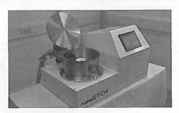
During operation, the nanoETCH supplies process gas (Argon, Nitrogen, Oxygen, Tetrafluoromethane) through MFCs. These, along with all other hardware, are controlled manually or automatically (recipe-based) via the touchscreen HMI.
