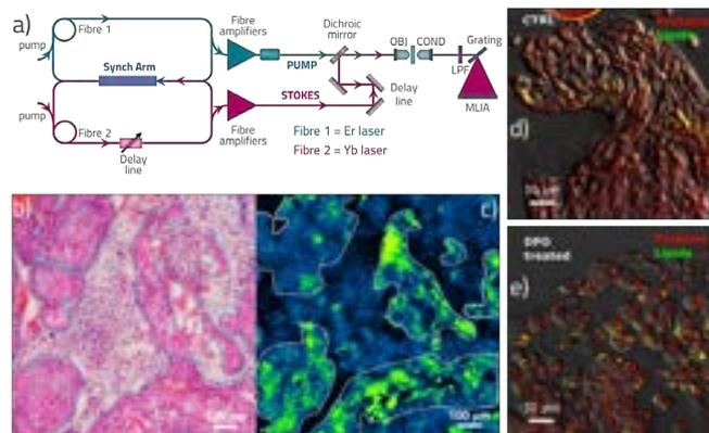
**Fig. 1** (a) System architecture. PPLN: periodically poled lithium niobate crystal; OBJ: objective; COND: condenser; LPF: low-pass filter; MLIA: multi-channel lock-in amplifier; (b) Image of human head and neck tumor tissue obtained with standard H&E staining and SRS microscopy at 2945  $\text{cm}^{-1}$  proteins peak (c) of adjacent tissue slices. HepG2 cells imaged with SRS microscopy (d, e) (grey brightfield, red proteins, green lipids) treated (e) and not treated (d) with DFO drug.
