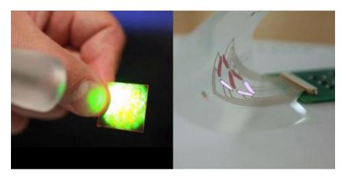
The prototype laser detection device, which can be used to protect goods against counterfeiting. Right: Printed electronics enable flexible, digital displays which can be bent without breaking. Credit: Nick Saffell
